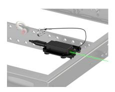
The LASER MAGPLATE facilitates vertical (tilt) adjustment of line arrays. It enables users to mount and dismount securely the TEQSAS LAP-TEQ PLUS laser inclinometer onto L-Acoustics' flying frames without any tool. Four magnetic pods attach the laser inclinometer to the support plate of the L-Acoustics flying frames, the K1-LASERMOUNT or K2-LASERMOUNT. Two alignment screws ensure correct positioning of the laser and a safety sling secures the laser to the flying frame or cabinet.
